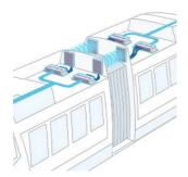
Wireless car-to-car coupling: Reliable and continuous connection, regardless of train composition, ensuring a secure and redundant onboard network.
